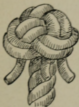
FIG. 126.—Double wall and crown.
